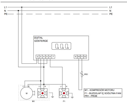
M1-COMPRESSOR ENGINE F1-REFRIGERATOR INTERNAL COOLING FAN PR1-PROBE
